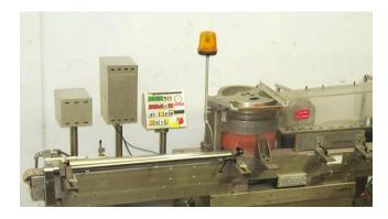
Packaging equipment used to have electromechanical controls with lots of buttons, relays and stuff.
