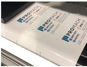
The Genesis printer can print the complete package, immediately before forming, filling and sealing the finished stickpack
